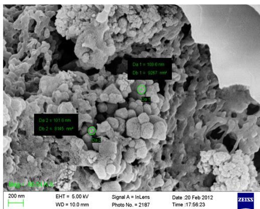
Figure 2: Scanning electron micrograph of BSA Np-QT
