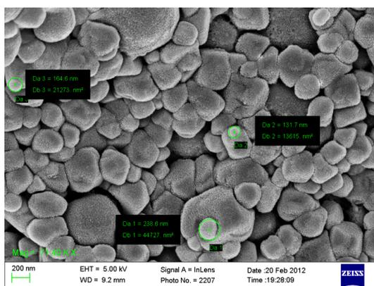
Figure 1: Scanning electron micrograph of BSA nanoparticles
